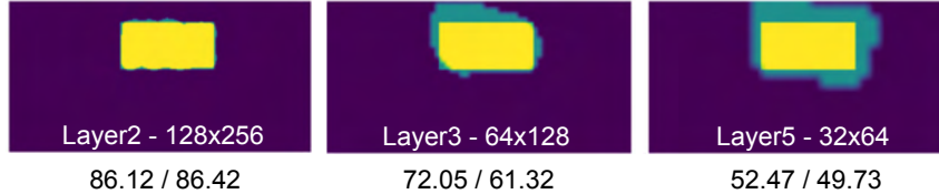
Figure 5.21: Mask-IoU (in black) for the digital adversarial patch with \beta = 0.6 and 0.8 on attacked cityscapes video using the ACAT_{GT} on different layers of DDRNet. The figures show the overlapping between the predicted mask and the ground truth for \beta = 0.6 , with the highest color indicating the degree of overlap. The depth of the DDRNet layer and the spatial dimension are denoted in white.
