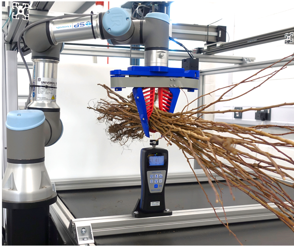
Fig. 14. The experimental setup for measuring the grip forces.
