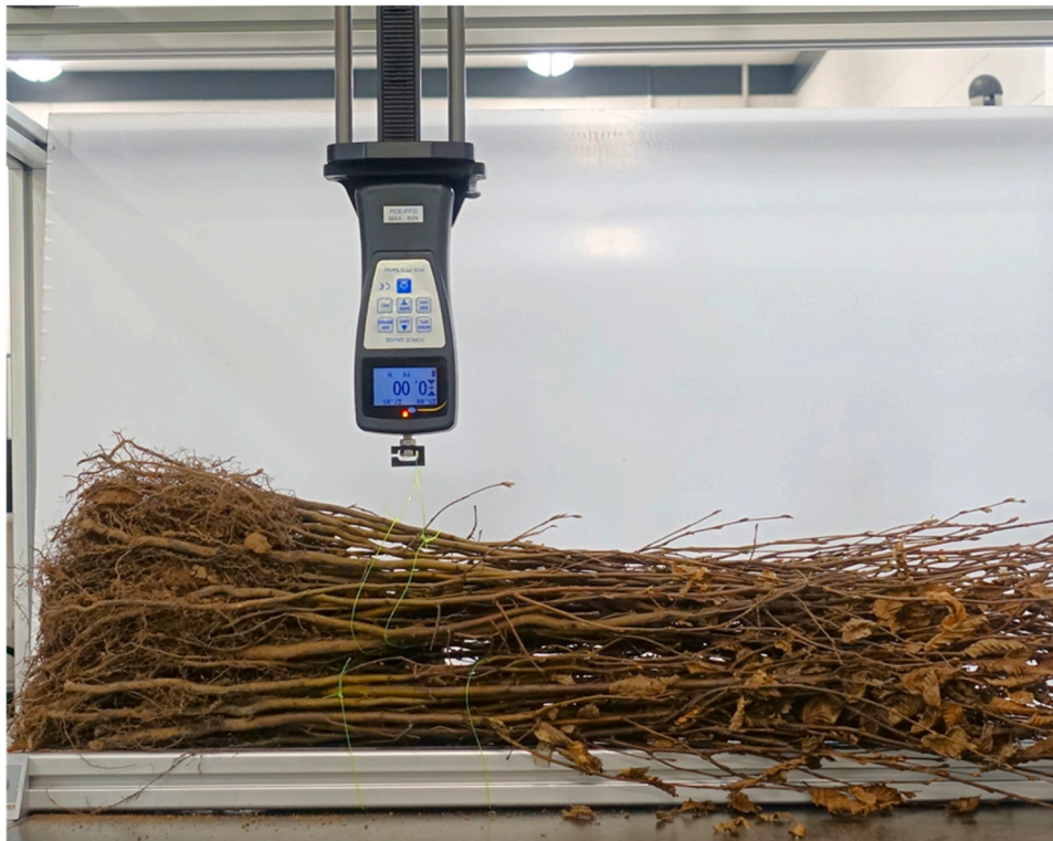
Fig. 12. The experimental setup for measuring the separation forces.
