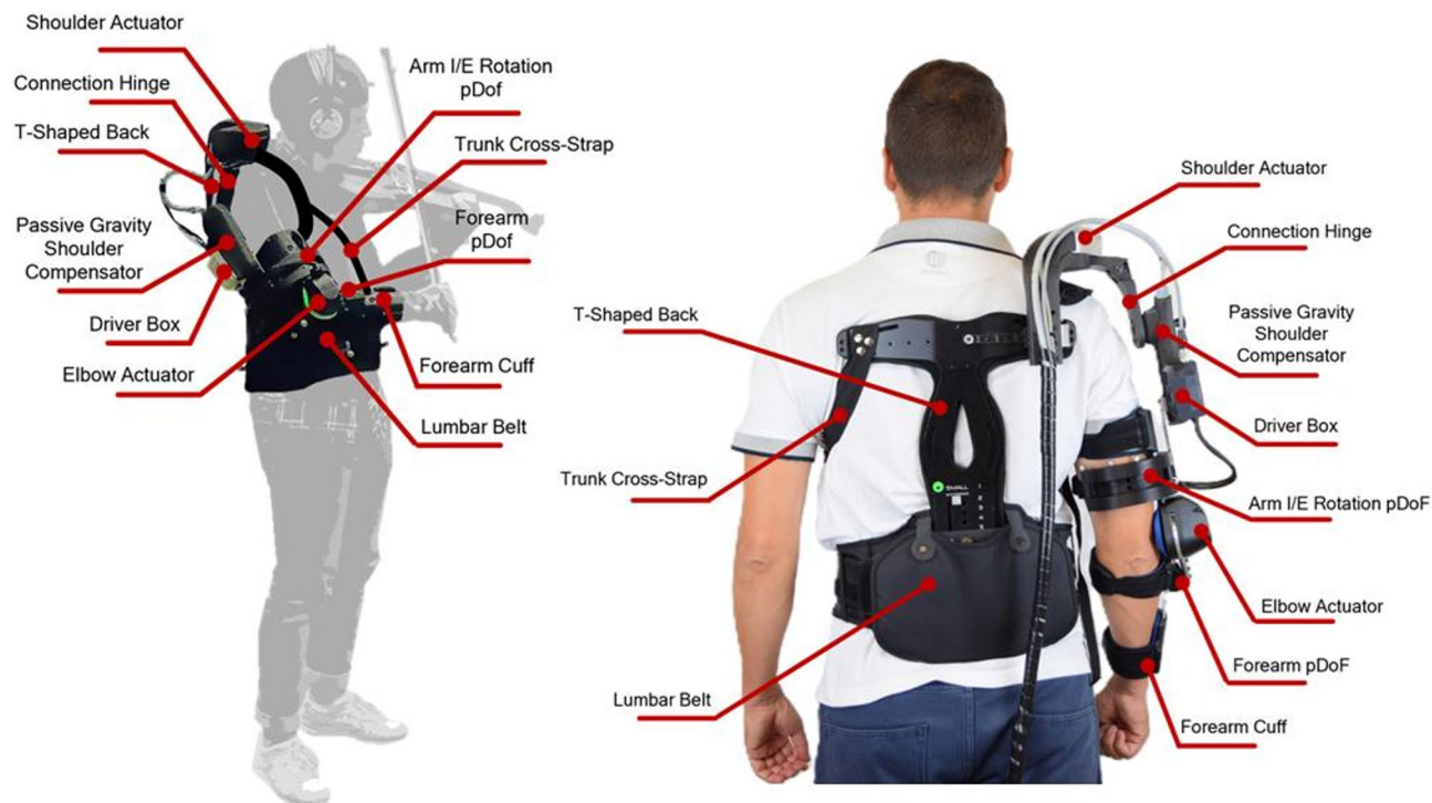
Fig. 1. Two views of the exoskeleton, consisting of the shoulder module and the elbow module. The actuators and the passive unloader are hosted in 3D printed parts, connected to a carbon fiber T-shaped frame. The active components are connected through a lockable hinge anchored to the passive shoulder gravity compensator. The overall structure is attached to the user's body through three main anchoring points: the semi-rigid lumbar belt, the trunk cross-strap and the arm and forearm cuffs, all using Velcro attachments to enable fast and easy donning/doffing and adaptability to different anthropometries. Finally, the passive internal/external (IE) rotation joint allows the physical connection of shoulder and elbow modules and the decoupling of their movements.
