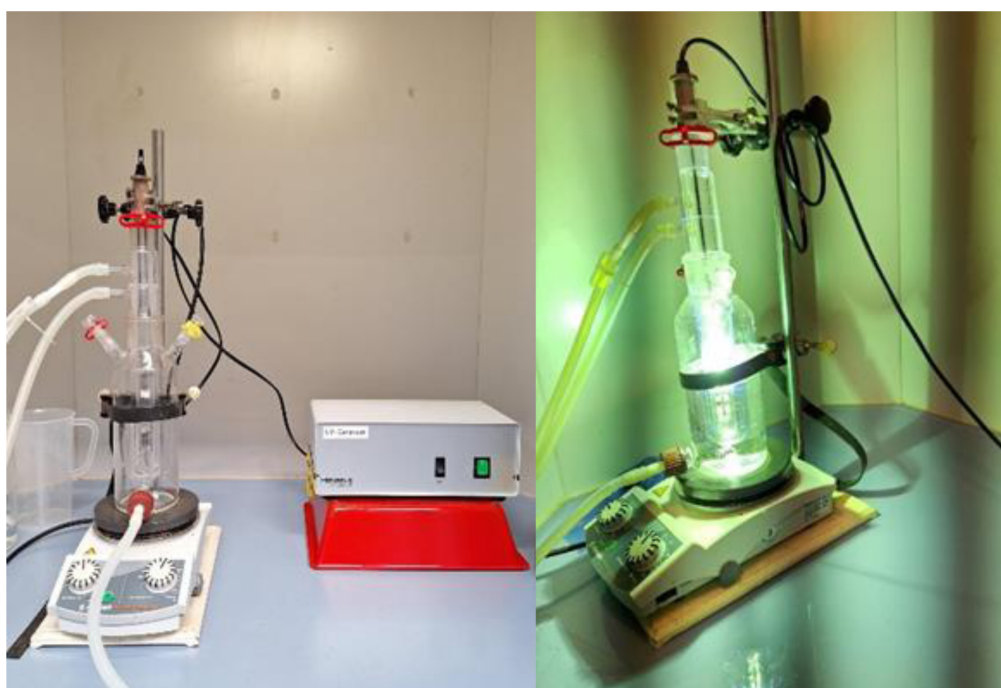
Fig. 3. Experimental equipment for oxidative degradation with \text{H}_2\text{O}_2/\text{UV} (left) and UV reactor with radiation source switched on (right).
