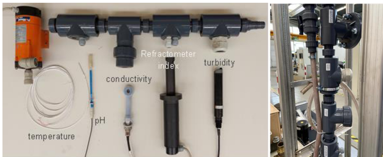
Fig. 2. Sensors used for the monitoring system in pilot trials (left), Connection of all sensors together using adapted fittings (right).
