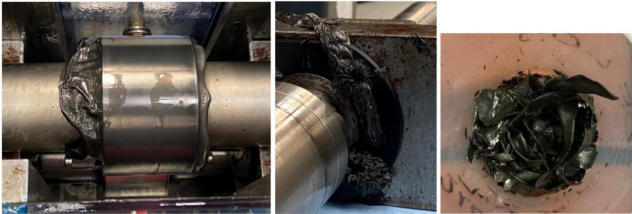
Fig. 5. Left and middle: Solid residues observed on the edges of the rolls at the 3-rolls test bench (OFL 03), Right: residue collected and analyzed afterwards with EDX methodology.
